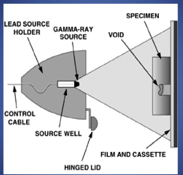
Gamma sources are normally more portable than x-ray equipment so have a clear advantage in certain applications, such as in remote areas. For remote area applications, the radiation source (Ir-192 or Se-75 in this case) is cranked into position and exposed to the area being tested.
