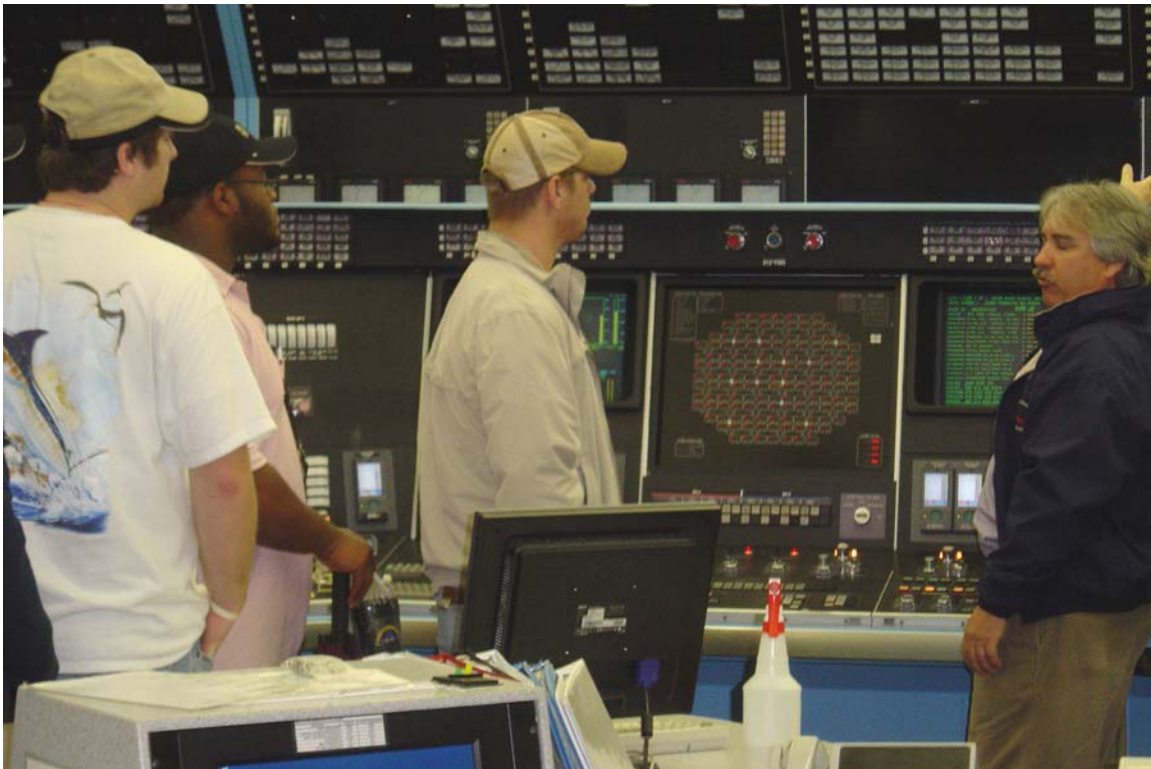
Photo in control room simulator. (with Dan Forman, James Hankins, and Jonathan Rogers; red dots mean full in rods for this scenario.)
